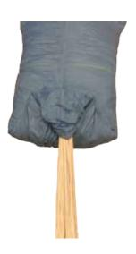
With one hand holding the rolled tail seam fold canopy back toward container without removing underneath hand.
