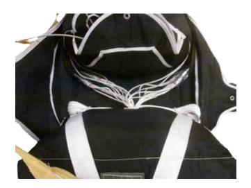
Seat the bottom of the bag in the pack try and push the top corners of the ALS bag into the top corners of the main pack tray so that the ALS bag is laying flat.
