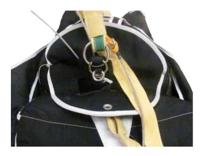
Lock in place by running the through loop around the small ring and back through the grommet on the drogue riser.
