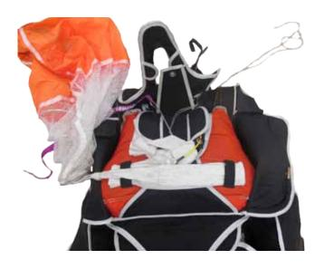
Route pull up cord up from the bottom and out through the top of the pilot chute. Make sure that pull up cord goes through the center of pilot chute spring.
