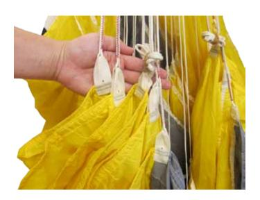
In order to soften the openings on new canopies you can roll the nose. After the canopy is broken in there is no need to do anything with the nose. Let it hang down naturally, grasp it and push it into the canopy folds a few inches.
