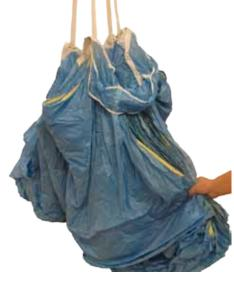
**4.4.3.11** Roll the leading edge three times (one and a half complete turns) to close all cell openings.
