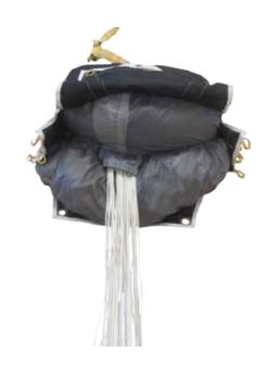
Make your first line stow by bringing the center inner rubber band up through the center grommet.
