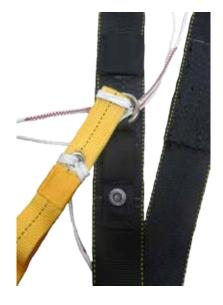
**4.7.2.5** Stow in elastic keeper located on riser.
