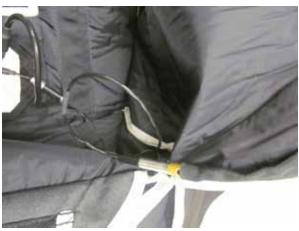
**4.3.1.12** At end of channel route cutter through elastic keeper.
