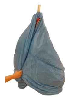
Hold the lines with one hand, the rolled tail with other hand and place canopy gently on the floor with rolled edge to the floor. Make sure that lines stay tight and canopy stays neatly rolled.
