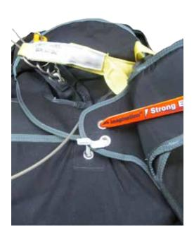
Close the left flap by bringing the pull up cord through the uppermost grommet on the left closing flap and pulling the closing loop through.
