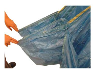
Gently pull each line tab towards the canopy to remove excess slack from lines. Once clear all "A" line tabs should be lined up evenly.
