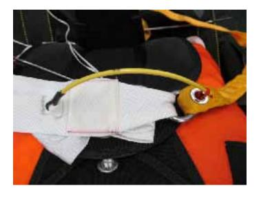
Open the right cover flap and insert the nylatron tab from the Air Anchor into the channel located under the cover flap.
