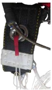
**4.6.2.6** Lock in place using the cutaway cable.
