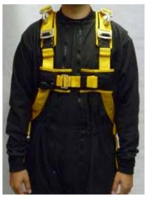
3) Fasten bellyband so chest strap and bellyband are equally snug. The main lift webs should be parallel from shoulder to hip.
