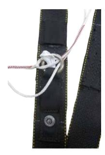
**4.7.2.4** Insert the tip of the toggle through the locking loop.
