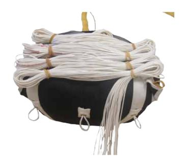
Stop stowing suspension lines when within about 4 feet of the links.
