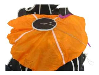
Roll material from right and left sides in to wrap around spring.
