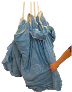
**4.4.3.12** Gently insert the rolled nose into the center of the canopy.
