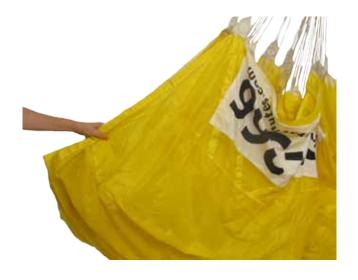
While controlling "A" line groups gently pull "B" line tabs to remove excess slack from lines. Then flake material between line groups to the outside.
