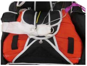
Lay the Air Anchor on top of the bridle with the red locking loop and nylatron tab facing up.
